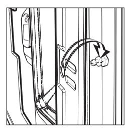
■ Lift the front locating hole on to the guide pin behind the collar.
